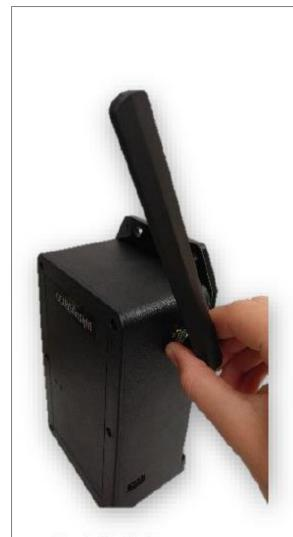
To fully tighten, move the antenna slightly anti-clockwise. Tighten the locking nut back up. Then holding the locking nut and antenna, rotate clockwise.
