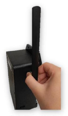
The locking nut should go tight and the antenna will lock in the location desired.
