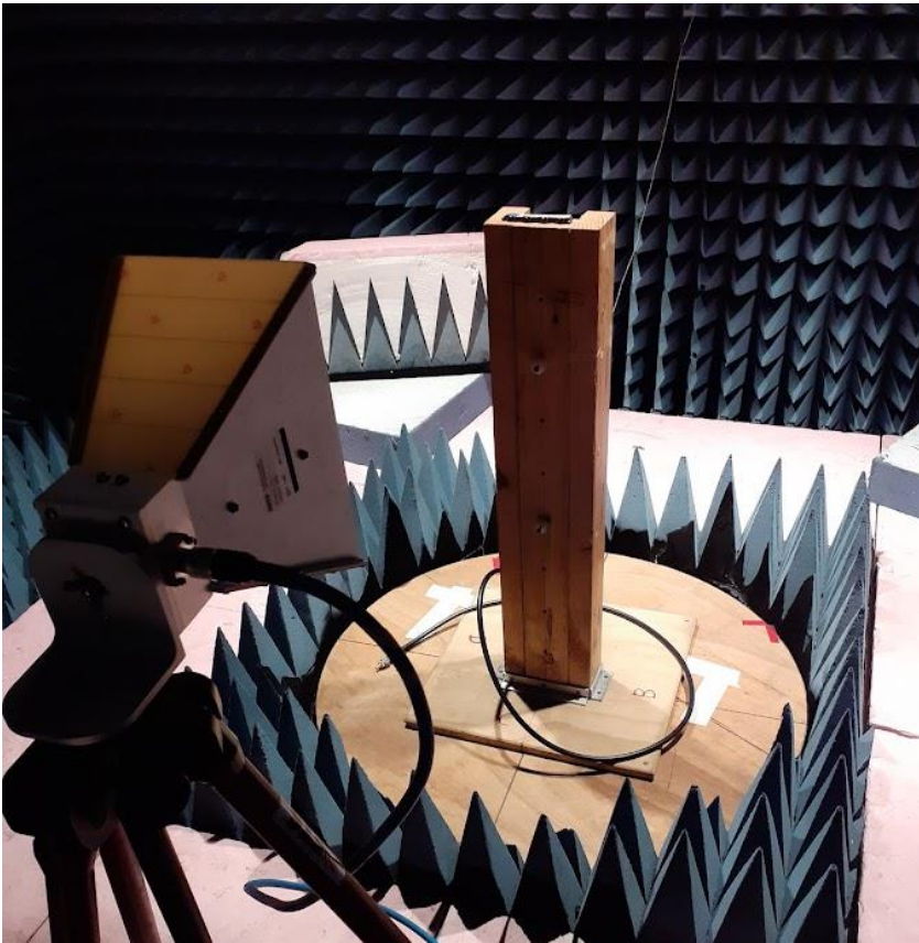
Figure 2 Photograph illustrating the measurement setup. The EUT is placed on top of the wooden pedestal. The EMC 3115 measurement antenna can be seen in the foreground.
