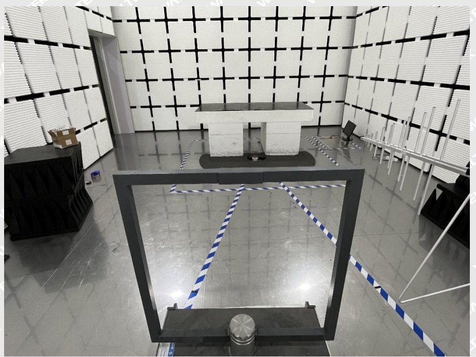
Radiation Emission Test Setup (Below 30MHz)
