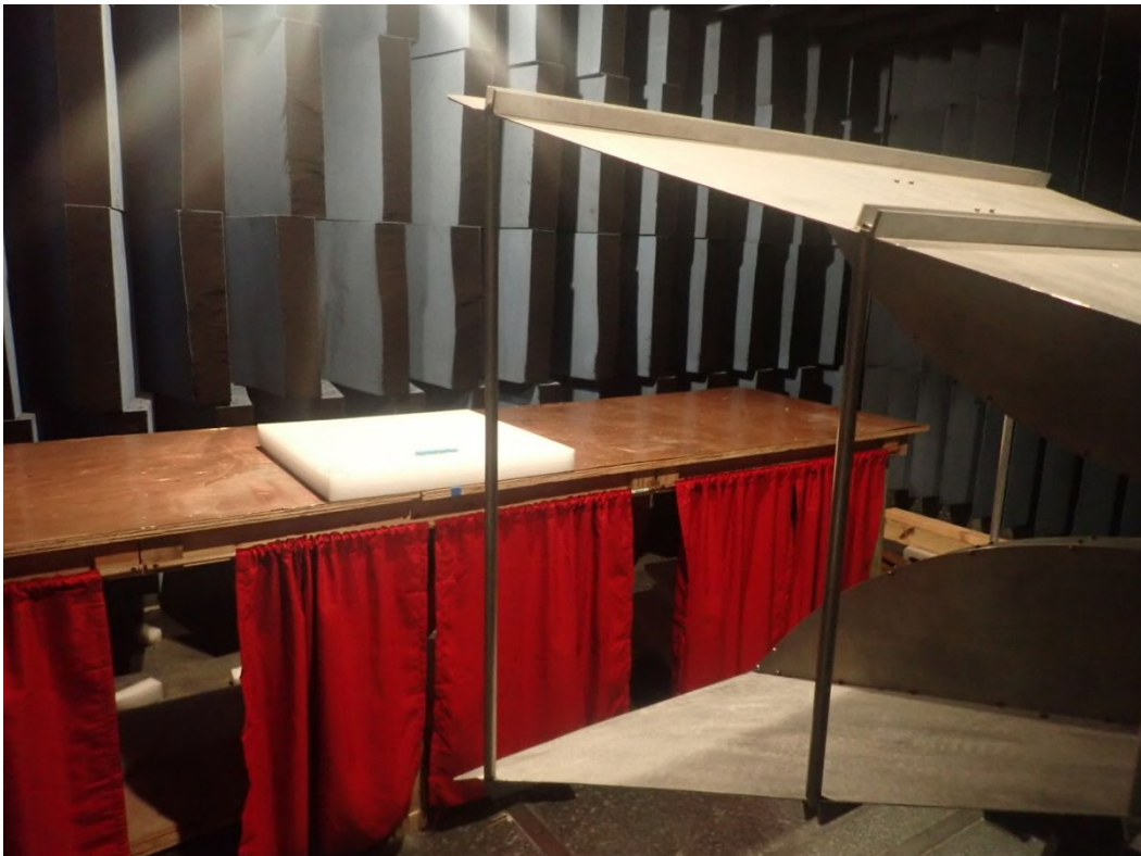
Section 21 RE Large DRG Antenna Test Setup, 200 MHz-1 GHz, Vertical
