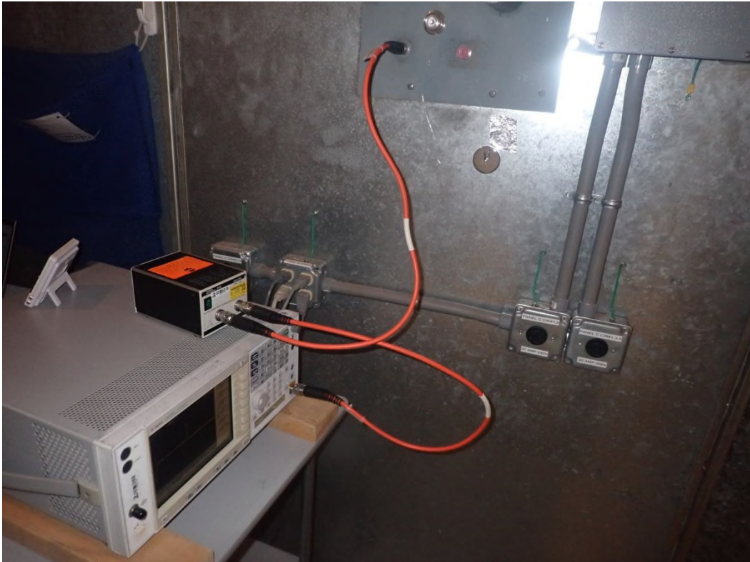
Section 21 RE Measurement Test Equipment, 100 MHz-1 GHz
