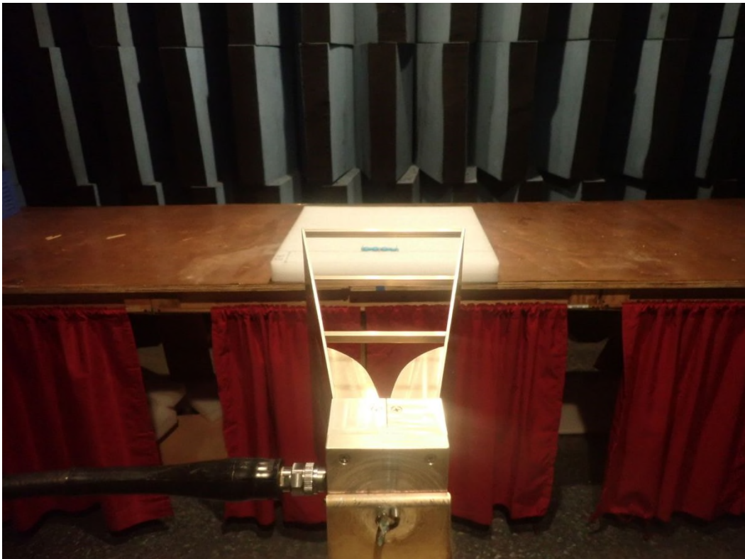
Section 21 RE Small DRG Antenna Test Setup, 1 GHz-6 GHz, Horizontal
